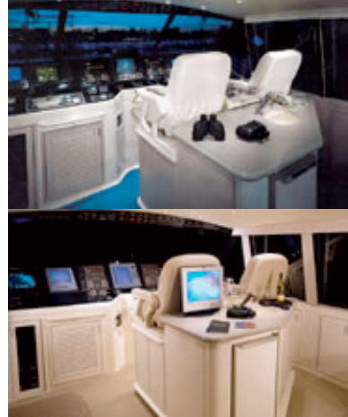
Bertram was among the first builders to offer an enclosed bridge for fish boats. During the refit, fresh carpet and upholstery were added, and the dash was altered to accommodate new electronics (bottom).
